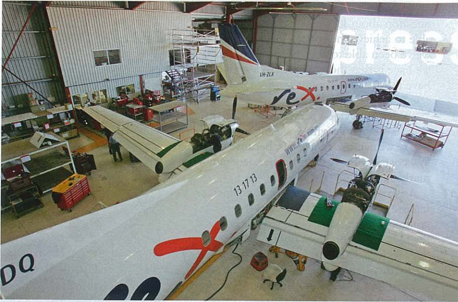
Inside one of Rex's maintenance hangars at Wagga. Saab 340B VH-KDQ (foreground) is undergoing a C check, newly arrived Saab 340B VH-ZLX is being prepared for service entry with the airline.
